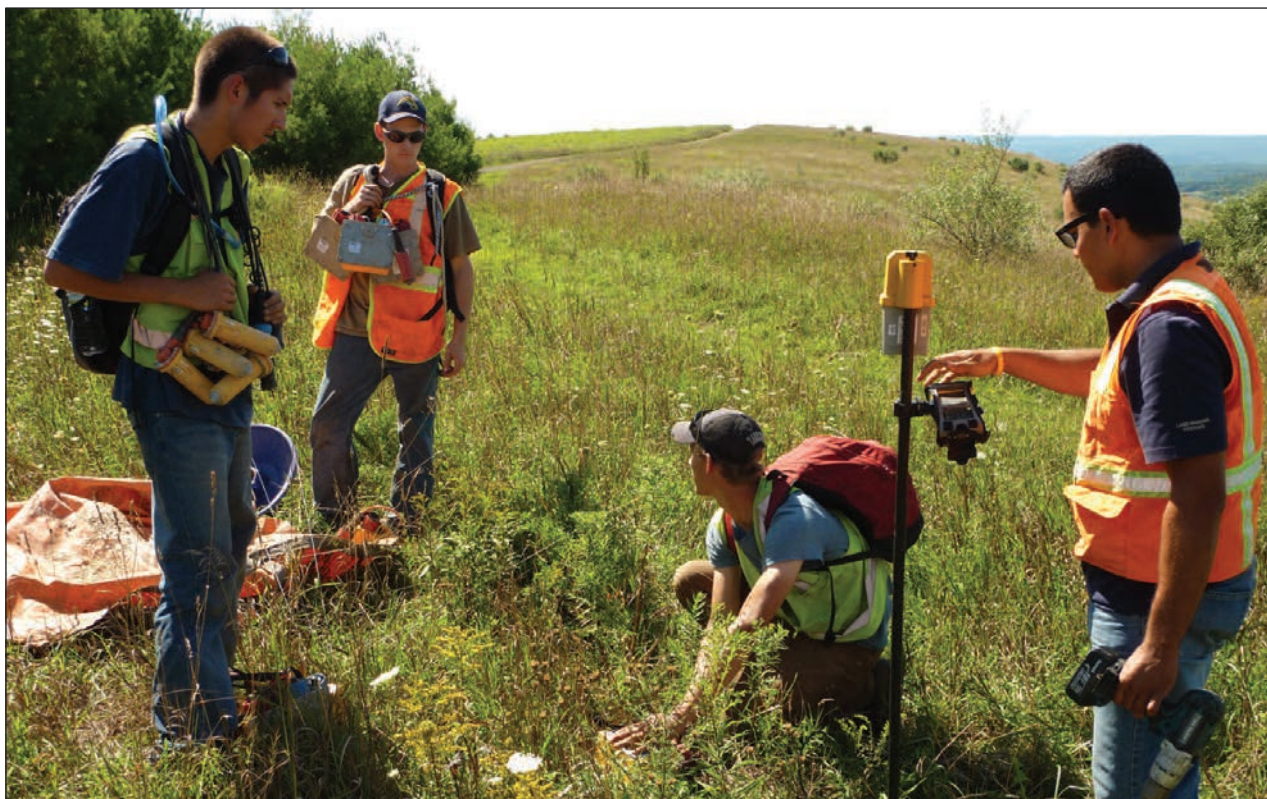
Crew members working on ION's ClearfieldSCAN program in the Marcellus shale play deploy INOVA FireFly and VectorSeis stations using the Connex operational management tool. (Photo courtesy of ION)
