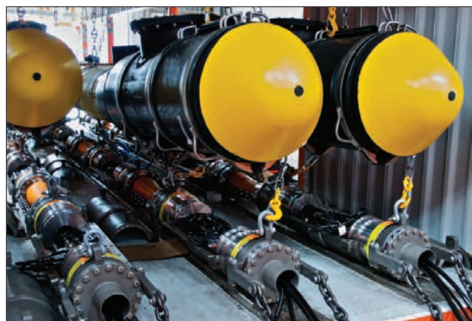
The PMSS source system enabled a quick retrofit of a non-seismic vessel. (Photo courtesy of WGP Exploration Ltd.)
